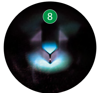
Visual confirmation of Raman laser alignment in all modes
